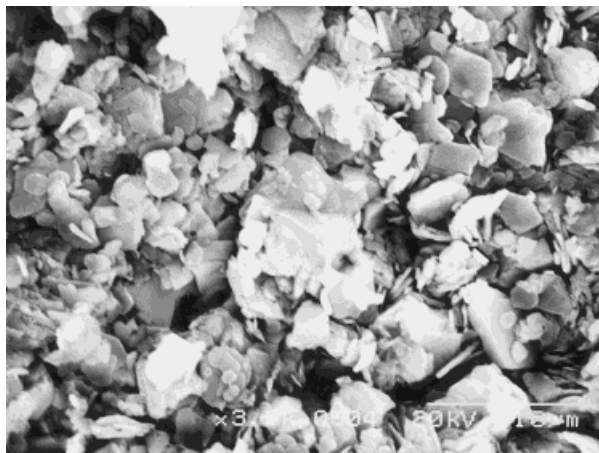
Figure 1 Scanning electron micrograph showing the platelet morphology of ZP powder.
